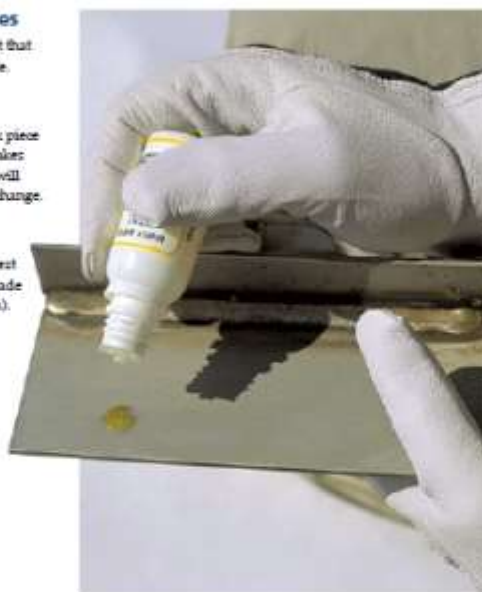
Easy identifying of stainless steel grade with Avesta Moly-Drop Test 960.
