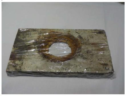
Aaron pointed out that in timber boats, it is not only the metal components that are protected by proper cathodic protection systems. He tabled a sample of a plank cut from a 75 foot timber boat that clearly showed the degradation around the skin fitting that had not been bonded in the protection system.
