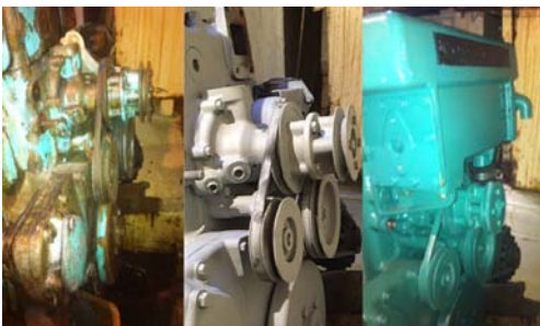
In the Engine Room, all the essential components were refurbished and painted including filters and heat exchangers.
