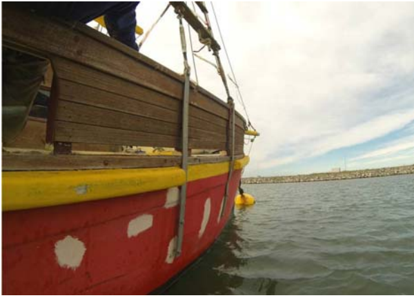
Following their purchase of Rose-F in 2015, Andrew and Jeremy replaced chainplates, rigging screws, bow roller and bob stay fittings and rigging in preparation for the trip from Bunbury to Fremantle.
