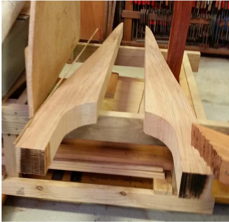
The components of a new set of jaws for a replacement gaff for Leeuwin await further work.
