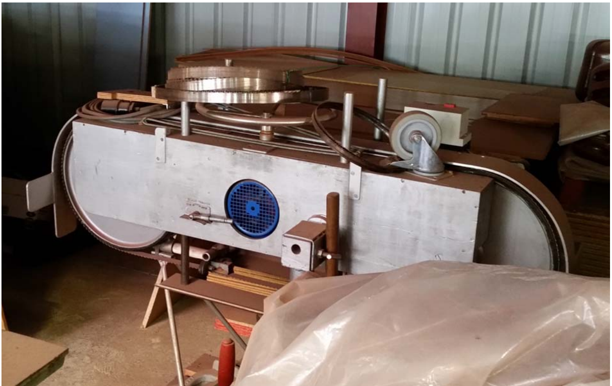
The mobile band saw designed and constructed by Ray Miller specifically to machine the corners and tapers on the large, long spars for the Leeuwin continues to be used for its original purpose.
