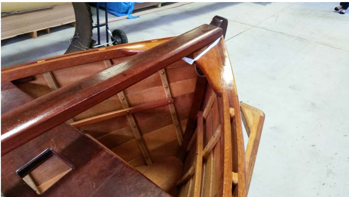
Further photos of Jack Tar showing the attention to detail that goes into the construction of a traditional clinker dinghy at the hand of professional boat builders who are masters of their art.
