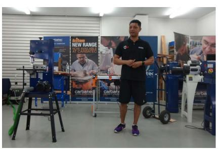
Garry began with a briefing and demonstration of a 10 inch Carbatec brand bandsaw. There is also a 14 inch version of this machine available. The 10 inch version is available at around \$480. Garry pointed out that the fitted blade had a greater number of teeth for profiling whilst a blade with a lesser number of teeth is available for ripping timber. Blades are available for between \$20 and \$30 each for this size saw.
