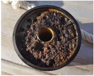
**Rob** also talked about finding cladosporium or some other microbial contamination in one of the fuel tanks as it sat around for the 5 years it took to rebuild the boat. The starboard tank was removed, cleaned, repaired and internally coated. This was all fine but the mistake was not doing the same for the port tank which was similarly contaminated and subsequently blocked the prefilter pictured on the right above.
