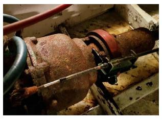
The quick fix 'she'll be right' solution is muffler putty but muffler putty does not work with steam around, so the exhaust leaks will soon be back again.
