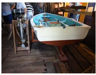
The major space within the boat shed was taken up by a clinker planked timber tender of the type that would have been built by the original boat building Cooper family and which Chris explained were used universally to access boats that were all on moorings prior to the time that jetties and marinas became the norm. There was also a late 1950's Fisherman model Seagull outboard that had reliably served the Mews family but still looked in remarkably good condition.
