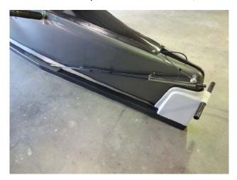
John has worked on the development of this new all carbon fibre design for several years and has now completed the build of the first boat which we were able to see at his factory. The main features of the new design are a fuller bow, more rounded hull and more rocker in the fore and aft direction.
