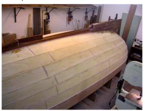
Nyata was used for the inner and outer stem, the bottom of the keel and the deadwood. Oregon was used for other framing. The inner and outer stem were laminated on the bench before being fitted to the boat at different stages of the process — the keel and inner stem prior to planking and the deadwood and outer stem later. A tongue and groove approach was used down the stem and in the deadwood components including the centrecase.
