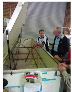
The whole mould is then placed in the oven to cure at 90-100 degrees C for varying times depending on the design and size of the moulding.
