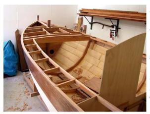
Following the usual excitement of seeing your creation upright and looking just like the boat you knew you were building, the deck and internal framing and fitout of the interior proceeded. This included the inwales at the gunwales, main deck beams, floors and the main plywood bulkheads together with bow and stern flotation bulkheads.
