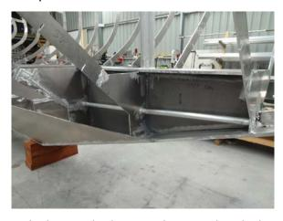
The framing out of the vessel includes a 9inch wide by 6inch deep socket on the deck to accommodate the bowsprit which will measure 2 metres clear from the boat. There is also a Samson post constructed from a 100mm diameter aluminium tube with a 10mm wall thickness. At the other end of the 'ship' Ed explained how he had modified the stern post and transom design so that a trim tab could be fitted in a practical manner.
