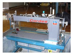
Here Pete gave us some practical advice about tension setting for these machines with particular reference to the bobbin. The tension on the bobbin spool should be set so that if one holds the bobbin vertically on the end of the thread, the bobbin should just fall under its own weight.
