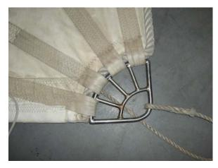
Notable in the fittings department was the clew iron, a large fabricated stainless steel frame that is sewn into the clew of sails too large for normal Rutgerson eyes or brass ferule type eyelets mentioned earlier.
