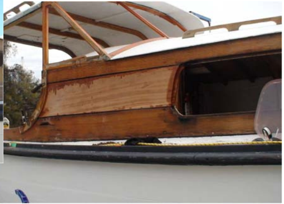
Rot in the cabin sides being cut out and replaced
