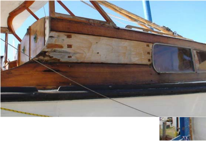
Rot in the cabin sides being cut out and replaced
