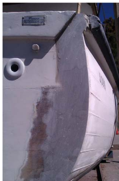
Rot in the transom and aft plank ends
