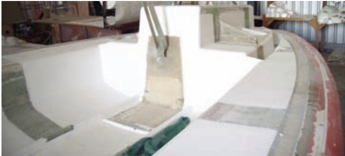
Close up of the rear deck lifting point, presumably to be cut off later.
