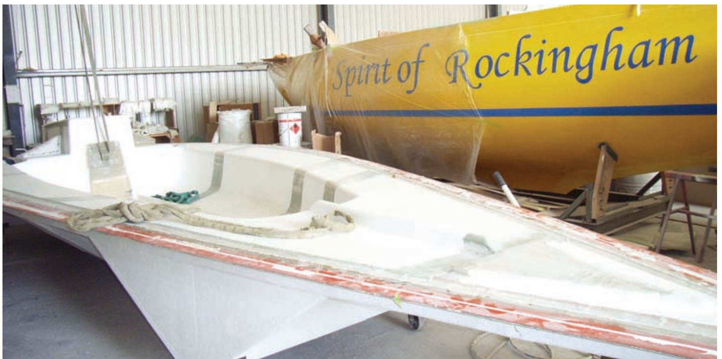
The S&S deck, still inverted in its mould, beside the hull.
