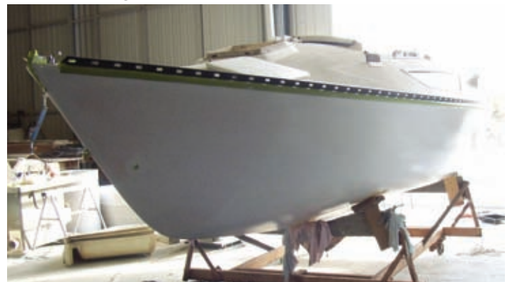
An older technology - Cameron and Hill Sorcerer of about 30 years ago, in for surface repairs, no doubt including osmosis treatment.
