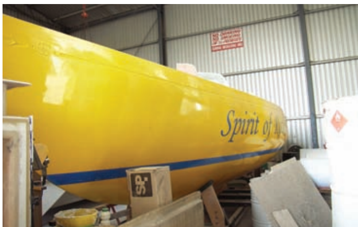
The undecked hull of "Spirit of Rockingham"
