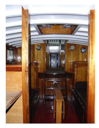
The half bulkheads at the foot of the bunks in the sleeping cabin were replaced by routered plywood to imitate the original tongue and groove jarrah. On re fitting, it was found that the old bulkheads were not plumb, and that filler pieces had been added to the bunk framing to disguise the gap.
