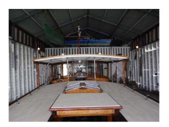
The problem was that the new ribs could only be fed between plank and stringer from above, which entailed removing not only the covering board at the perimeter of the foredeck, but also all the after deck fittings, rubbing stakes, canvas sheath and securing beads etc.
