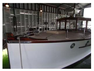
Nokomis is planked with kauri pine riveted to karri ribs on a jarrah keel. Where possible the inside half of the laminated ribs continued from gunwhale to gunwhale. The decks are of oregan pine nailed to their beams, and the super structure is Queensland maple.
