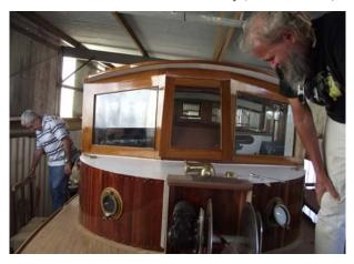
Out on deck, the quality of the workmanship that Ron and Kev have put in over so many months is in evidence everywhere. The teak laid deck and the external joinery and detailed cabinet work on the cabin are a masterpiece. And the 'jewel in the crown' is the turned timber stanchions and hood bows over the stern cockpit which will support a portable awning. Below the gunwales, Ron points out that he was able to retain all of the original timber in the hull, including the rubbing stakes.
