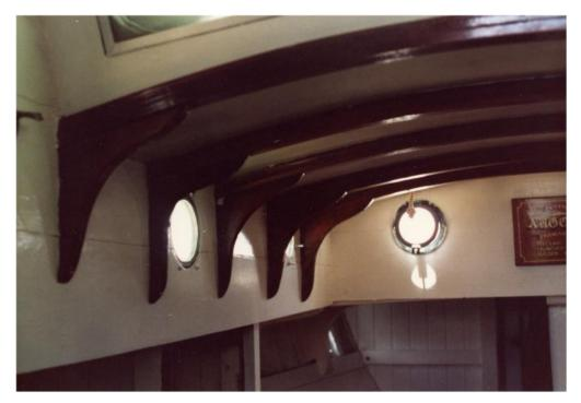
The 'look & feel' of the interior was very traditional but once again fresh water ingress had taken its toll and much of the structure was no longer sound. The limited camber built into the decks of these older vessels and their tendency to incur sagging of deck beams around the cabin trunk edges resulted in fresh water collecting along the trunk/deck joints leading to rot travelling into the cabin structure. Chris has retained much of the interior fitout as patterns for the rebuild.
