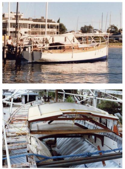
The next task was to remove the plank deck which was fixed down with large steel pins that had become entirely rusted and non existent. The cabin trunk and doghouse were then dismantled and removed, leaving Argosy at the same stage of construction as she had been during WWII.
