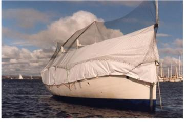
Early in the project , Chris obtained a mooring at Crawley Bay and manufacture of a frame from PVC pipe and a vinyl cover to keep the fresh water out took on the form of a significant subproject. This included nets and other patented devices to keep the birds off. Scraping, sanding and dismantling of the hull interior continued at the mooring.
