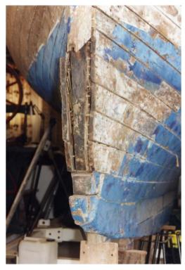
Prior to work ceasing in the mid 1990's, Chris commenced work on the stem post, removing the degraded fixings in the plank ends with a view to replacing the stem post before re-fixing the planks. This remains 'work in progress'.
