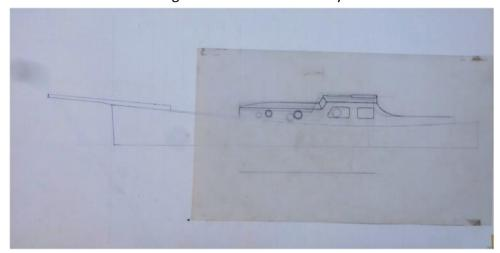
However, Chris would prefer to maintain the single level trunk as she was at launch. Additional headroom can be achieved by adding a narrow plank above the current gunwale line and increasing the deck camber to the side of the cabin. Two slightly different drawings of this arrangement are shown below.
