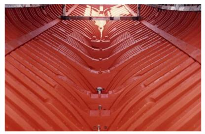
Following the completion of the 36 ribs, each of which covered 6 planks, the scraping and sanding of the entire inside of the hull up to the first stringer down from the gunwale was completed. A liberal coating of Cupronol (no longer available) was applied before all surfaces were painted with Epicraft red lead, followed by Epicraft white undercoat and one gloss topcoat. She then returned to the water in much sounder condition.
