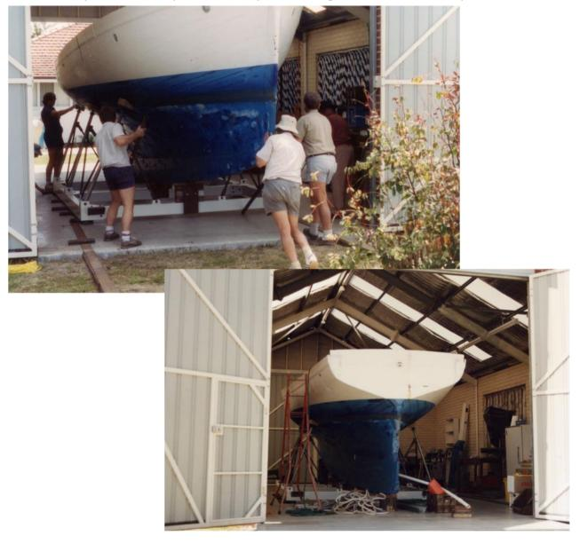
Chris, together with helpers Don and Mike, spent subsequent 'work days' burning off the paint on the topsides and stripping out the caulking. The topsides have largely been sanded up and fixtures such as the portholes in the bow removed.
