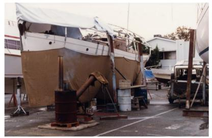
On Friday 16th September, 1988, Argosy was lifted out of the water for an extended period of time on the hard. Although it was winter, hessian was draped around the hull to limit the drying out of the planking. A 44 gallon drum was used to provide the fire power for the steam box with a blanked off piece of bore casing serving the purpose as the water/steam bath.
