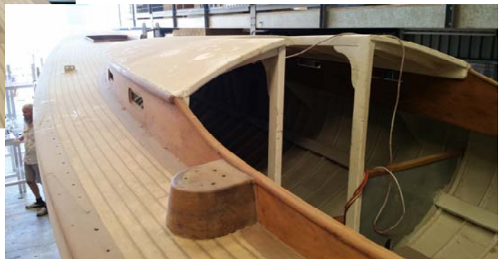
Note the good crown in the top of the original coach house which creates some room (but not standing room) inside the narrow 7 foot beam hull.
