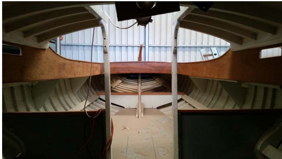
“Joyous” - The view forward (above) and aft (below). Note the knees and beams in lieu of a kingpost under the mast
