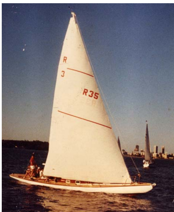
1970's, "Flame" with mast head rig and large genoa.
