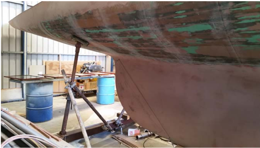
“Joyous” aft sections and the completed replacement rudder to the original design.
