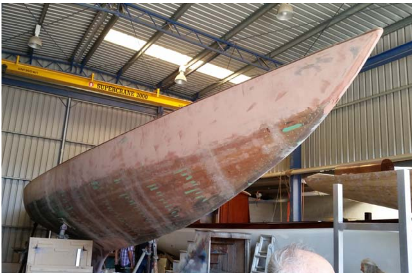
“Joyous” long sleek hull glassed and ready for final fairing.
