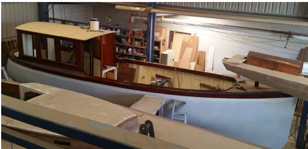
"Vectis" showing the open cockpit area forward of the enclosed aft cabin and below the high, plumb stem, fine bow and substantial freeboard
