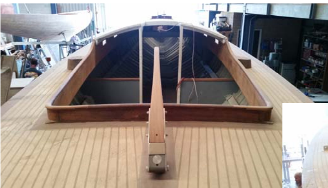
Note the good crown in the top of the original coach house which creates some room (but not standing room) inside the narrow 7 foot beam hull.
