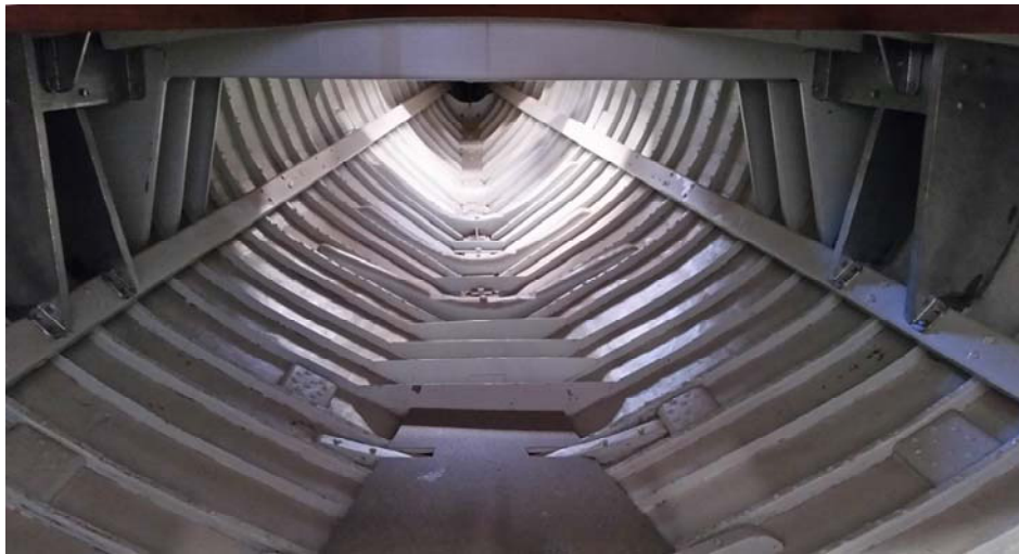
“Joyous” - The view forward (above) and aft (below). Note the knees and beams in lieu of a kingpost under the mast
