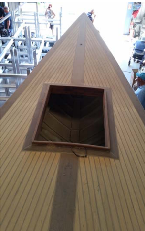
Geoff Leggatt admiring the sprung deck on “Joyous”. Her narrow ends and the good original condition of all the deck fit out other than the beech deck itself are evident.
