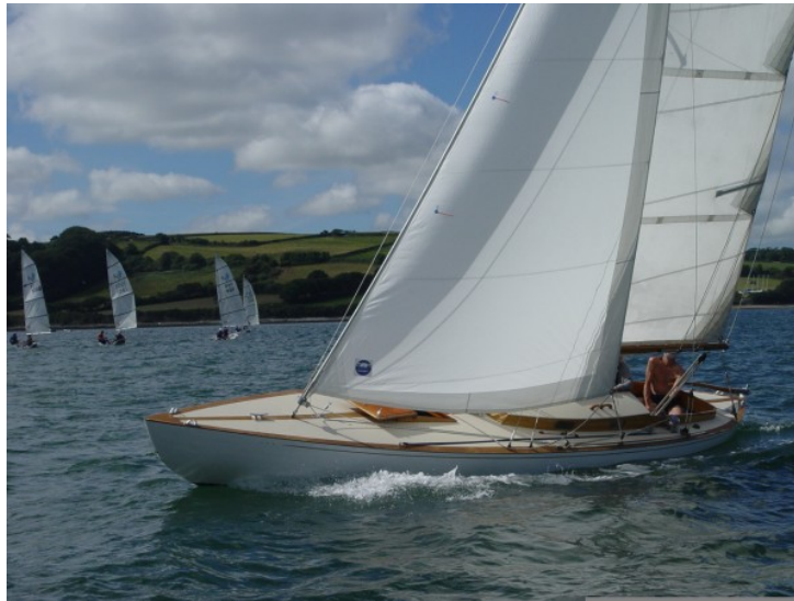
A sister ship on the wind, the fine bow 'cutting' the water with little disturbance.
