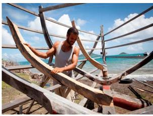
The hull shape was taken from a half model based on generations of experience. The building process commenced with the fast growing West Indian White Cedar being cut from the local forest for framing. The timber was worked using the adze and the levels were taken using the natural level of the horizon – the framing being set up on the open beach at Windward. The vessel was to be 42 feet overall length with a beam of nearly 12 feet.
