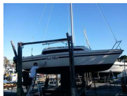
2 coats of Hempel antifouling applied to Light Primer. No evidence of applying an underwater primer before the antifouling. 4 years later the white Light Primer was clearly evident but little or no black antifouling remained. I believe that an underwater primer is required to get the antifouling to stick to the Light Primer epoxy.
