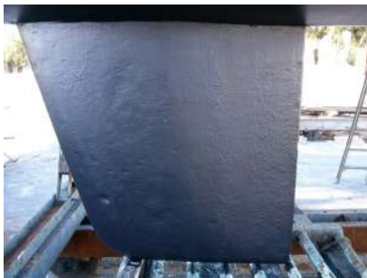
2 coats of Hempel antifouling applied to Light Primer. No evidence of applying an underwater primer before the antifouling. 4 years later the white Light Primer was clearly evident but little or no black antifouling remained. I believe that an underwater primer is required to get the antifouling to stick to the Light Primer epoxy.
