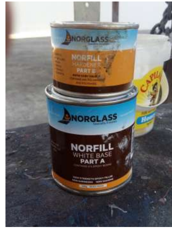
2 coats of Hempel's Light Primer was applied to the keel. Norglass Norfill was used to fill any divots and create a fillet where the keel joins the hull. The back of a metal teaspoon was used to form the fillet
