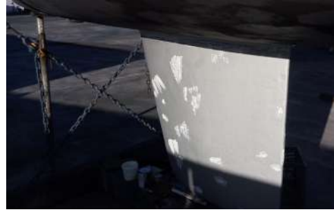
2 coats of Hempel's Light Primer was applied to the keel. Norglass Norfill was used to fill any divots and create a fillet where the keel joins the hull. The back of a metal teaspoon was used to form the fillet
