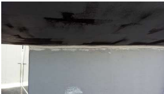
A coat of Hempel's Underwater Primer was applied. More fairing was done and primed over.
