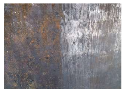
Keel ground back to bare metal using 4" angle grinder fitted with a metal grinding disc on advice from Gary Martin of Boat Paints. A slow and noisy task.
