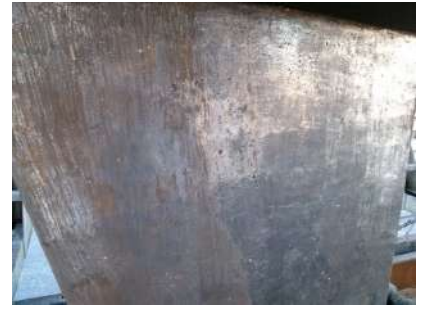
No time to use a rust convertor Some rust left in the deeper pits
