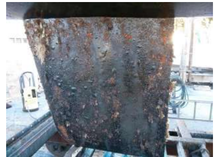
Many blisters present only a few years after being "professionally" treated
