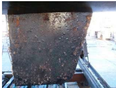
Many blisters present only a few years after being "professionally" treated
