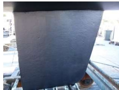
2 coats of Hempel antifouling applied to Light Primer. No evidence of applying an underwater primer before the antifouling. 4 years later the white Light Primer was clearly evident but little or no black antifouling remained. I believe that an underwater primer is required to get the antifouling to stick to the Light Primer epoxy.
