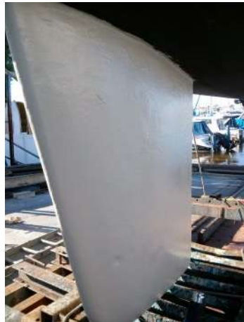
Applied Hempel two pack epoxy primer & undercoat directly to the shiny metal. ( Hempel Light Primer & Curing Agent 95360 Ratio 2:1) No time to fill and sand so some divots remained. No time to give keel to hull joint much attention so expected this to be a rust area next time boat was slipped.
