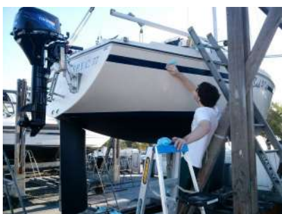
2 coats of Hempel antifouling applied to Light Primer. No evidence of applying an underwater primer before the antifouling. 4 years later the white Light Primer was clearly evident but little or no black antifouling remained. I believe that an underwater primer is required to get the antifouling to stick to the Light Primer epoxy.
