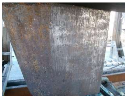
Keel ground back to bare metal using 4" angle grinder fitted with a metal grinding disc on advice from Gary Martin of Boat Paints. A slow and noisy task.
