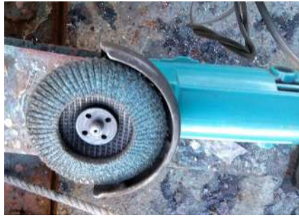
After removing most of the rust, grinding disc replaced with a sanding wheel to get back to shiny metal
