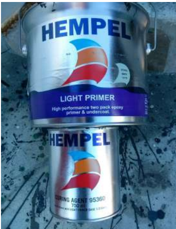
Applied Hempel two pack epoxy primer & undercoat directly to the shiny metal. ( Hempel Light Primer & Curing Agent 95360 Ratio 2:1) No time to fill and sand so some divots remained. No time to give keel to hull joint much attention so expected this to be a rust area next time boat was slipped.
