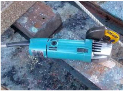
After removing most of the rust, grinding disc replaced with a sanding wheel to get back to shiny metal
