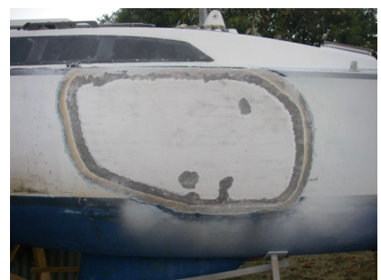
The start of filling and faring
