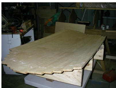
Mould removed, bought inside and faired
