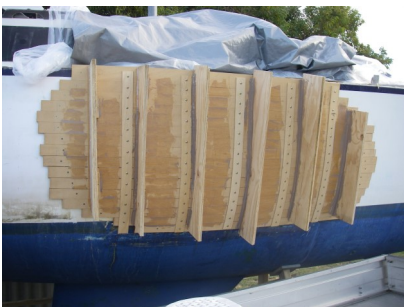
Stiffeners glassed in place
