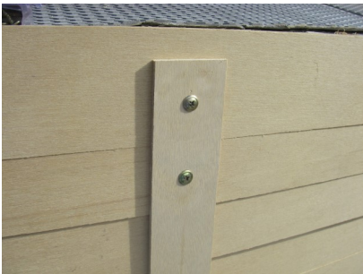
Vertical battens to form shape of hull
