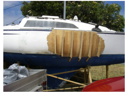
Prepared mould re-attached
