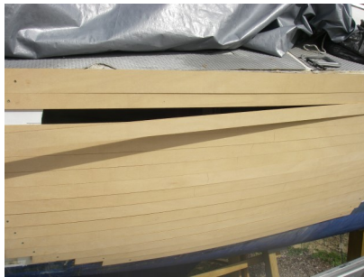
Strips marked and trimmed
