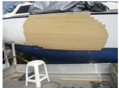
Strips kept horizontal for appearance if faring not good
