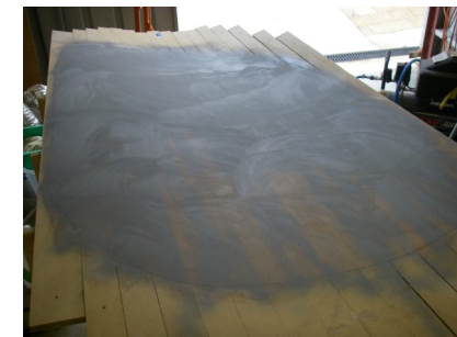
Wax applied for gelcoat
