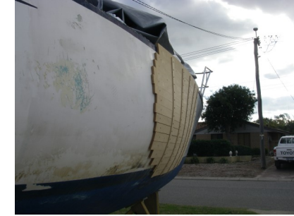
Strips kept horizontal for appearance if faring not good
