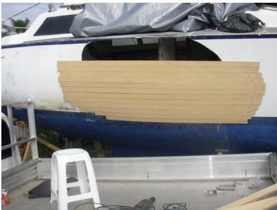
Ply strips screwed to hull
