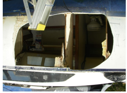
Initial cutback to sound fiberglass & feathered inside
