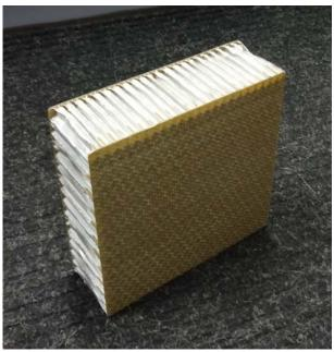
The simplest of these is Divinycell, a foam sheet material that is available in thicknesses from around 6mm up to several hundred mm. When used with a fibreglass layer each side this is a very strong material for general construction such as building a dinghy or super structure. Another alternative is Nomex, a honeycomb type material which bends well in one direction but is very expensive. For more complex projects there is X-Panel made up with corrugated aluminium
