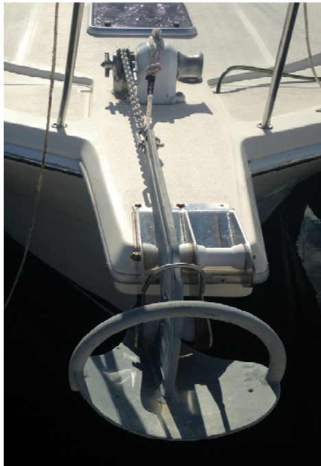
Horizontal Axis Windlass
