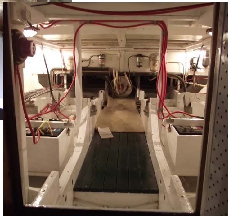
Karrawa - the engine room under the saloon floor looking aft. All restored and ready for the twin diesels to be re installed
