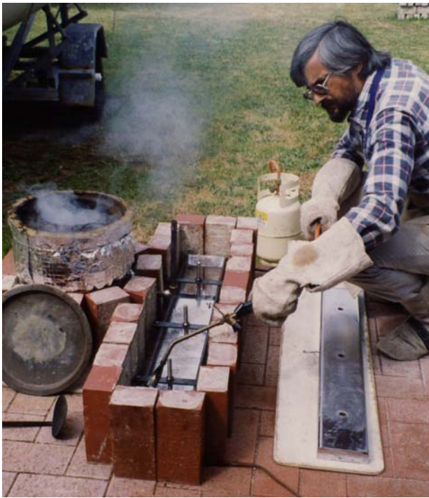
Melting the lead external ballast into a 150mm x 75 mm mould with a brick
