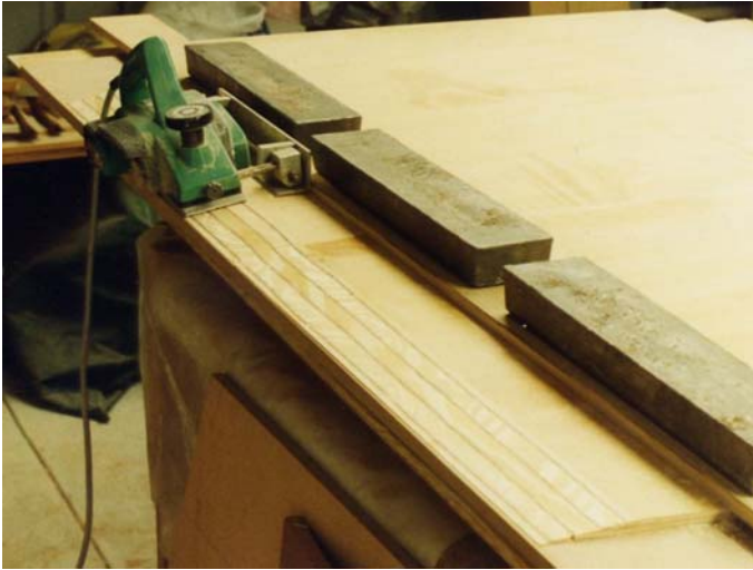
Using a planer angle attachment and straight edge to prepare plywood scarp joints
