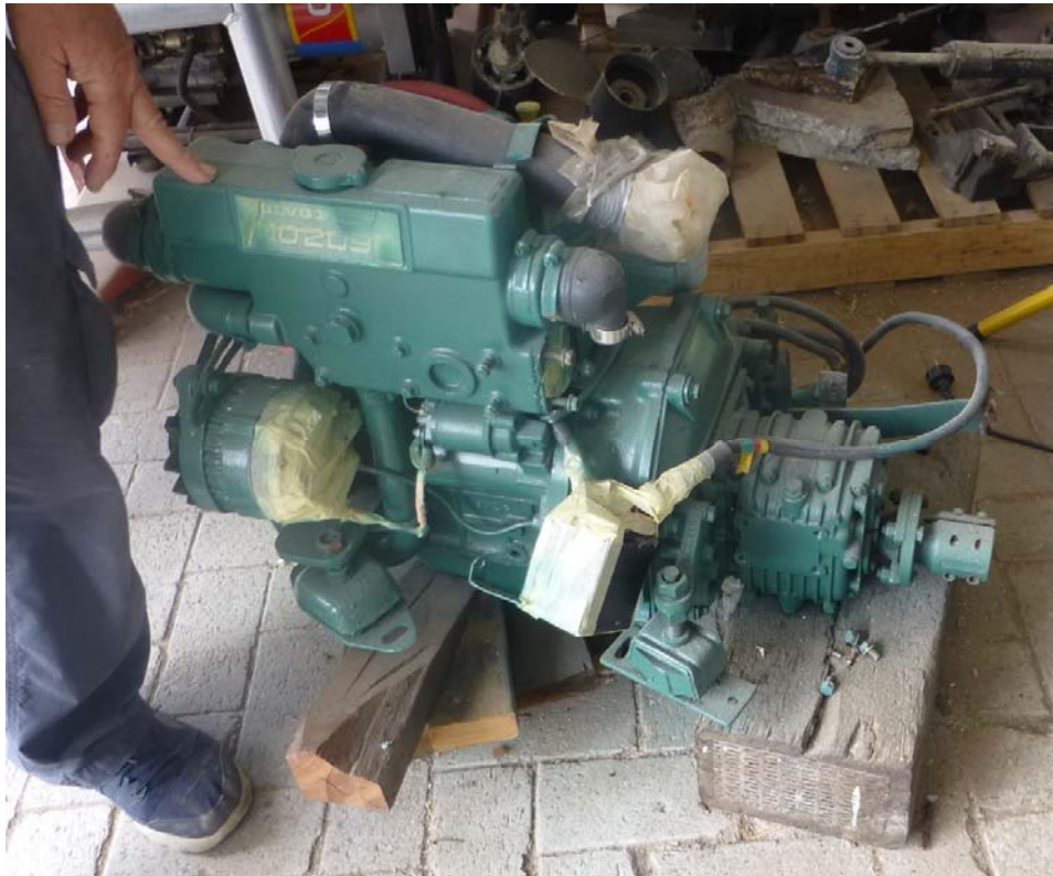
The 30 hp Volvo MD203 and Hurth gearbox pushes the vessel along at 8 knots.
