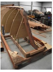
bolted on and sheathed after fairing. Stringers and the engine beds will also be fitted to the frames before planking. The first two planks of western red cedar had been fitted after convex and concave machining of opposite edges on Mick's spindle moulder with the new cutter head
