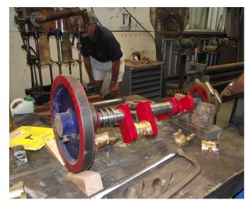
This is a compound engine with a high pressure cylinder of 4" diameter and a low pressure cylinder of 8" diameter to use the double expansion energy of the steam. Not quite as desirable as the triple expansion engine built for EMMAMADELINE but still very good and a popular compromise for bigger steam boats of the times.
