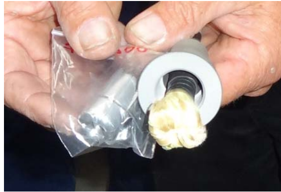
The sequence of applying a furling termination to a braided forestay
