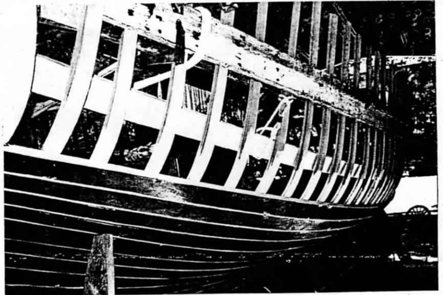
Every one of these ribs is new, and all the planks will be, also.
