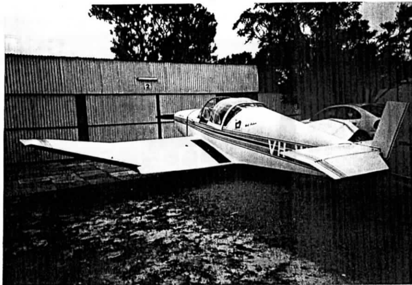
Wally Nilan's Bebe Jodell, now about 25 years old. Note the neat, turned up wingtips. 100hp Continental.
