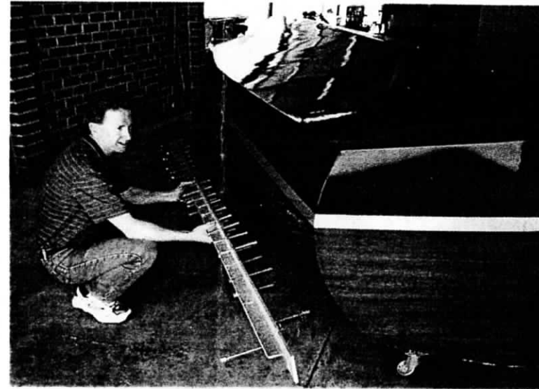
Andrew demonstrates device used for holding external skin strips in place when glued
