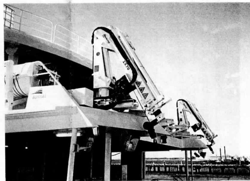
"True North's" two boat-handling derricks on the upper stern deck. They lift boats from either this deck or the lower one.
