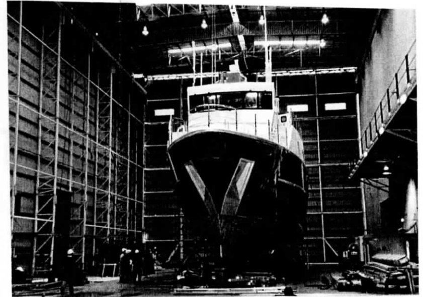
From the bow, the near-complete Work Boat-Style Yacht. Observe the huge anchor recesses. Small figures on left give scale.
