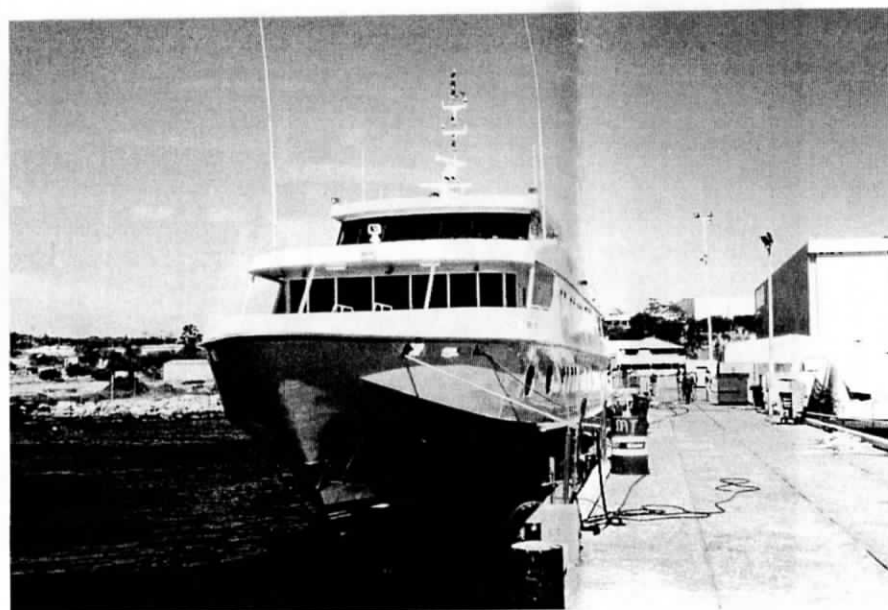
Accommodation and bridge, viewed from the stern. Two boats will go about here. Sikaflex still to be cleaned off most decking.
