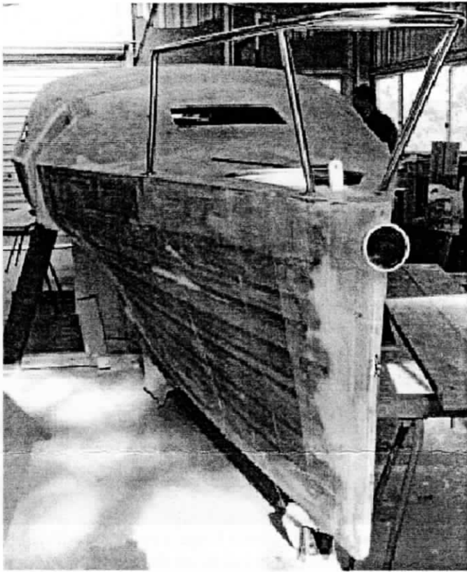
ABOVE: The fine lines of the Ferrier bow are clearly visible in this photo. Note the tube which houses the removable carbon fibre bow sprit.
