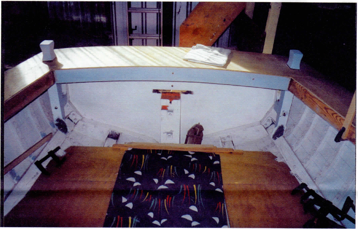
The generous cockpit almost complete. Will have a top over. Note Samson posts
