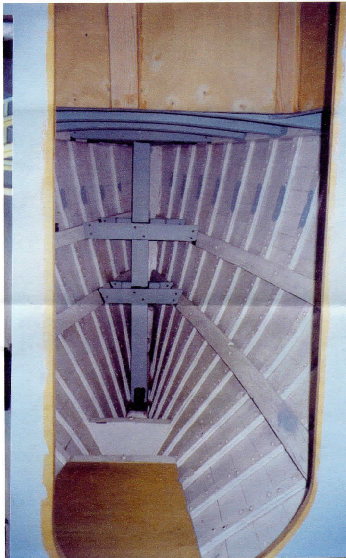
The forepeak, through the main bulkhead. Ribs are laminated.
