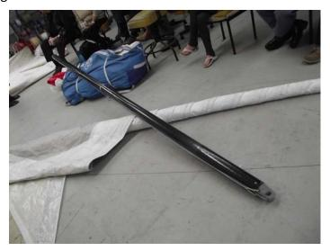
Despite all the modern technology, weight aloft can still be a problem. Modern materials can assist with solutions, for example a carbon fibre mast on a 44 footer is 90 kg lighter than its equivalent aluminium mast.
