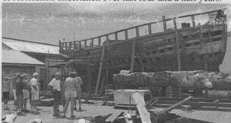
Photo 11: Old fishing vessel being reconstructed from a forest of Tuart trees
