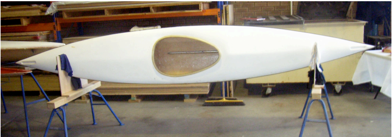
A kayak, side mounted, at Paul's for fastening of deck to hull
