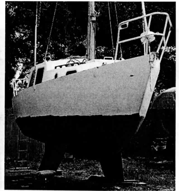
Photo 7: Multi chine steel vessel with bilge keels
