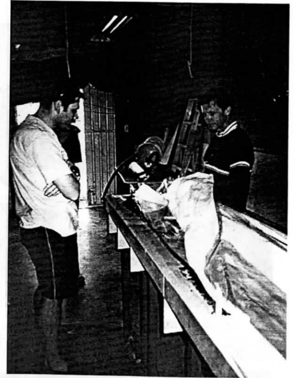
Geoff Leggatt and Kim Klaka examine the bottom end of the very large mast half in its mould.
