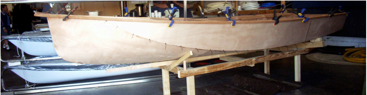
The 14' Sabre class monotype dinghy being built by Louis at Boating Hardware
