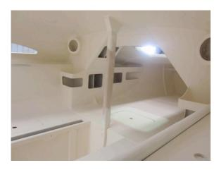
The monocoque-style construction has been enhanced by the integration of all hardware mounting and lockers within the interior. It's a super smooth finish - with non slip texture - where it's needed.
